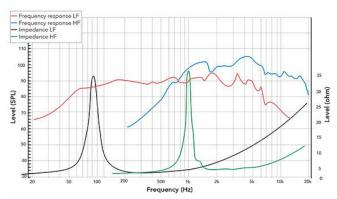
Frequency response measured on IAC baffle
